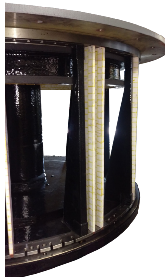
Figure 3. Close up of wear protection showing ALOX tiles and polyurethane coatings.
